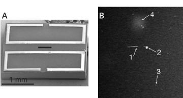
An SEM image of the GapSet E-chip used to form the microfluidic channel is shown in Figure A. Figure B shows a STEM image of nanoparticle flow. A series of streaks is visible at arrow 1, which presumably are due to a single gold nanoparticle moving to the left.
