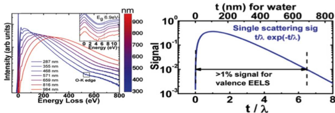
Figure 5: The left image shows the core- and low-loss (inset) components of the EELS spectra of water. The right image shows a simulation confirming the experimental findings. With a  $t/\lambda$  value of up to 6.5 low-loss EELS is generally meaningful.
