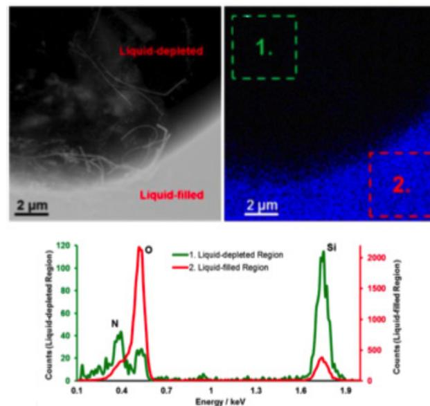
**Figure 8:** The top images are a STEM dark field image (left), and an EDS spectrum image (right) of the same area. The blue area on the right shows a larger volume of water present. The bottom image shows EDS spectra from region 1 and region 2 indicated in the spectrum image. In region 2 where water is present, oxygen dominates the spectrum.
