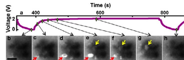
Figure 6: The TEM images show a charge/discharge cycle of a single group of FePO<sub>4</sub> nanoparticles. The EFTEM images (b-h) indicate where lithium is located spatially during the cycle.
