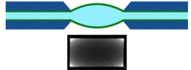
**Figure 2:** The top figure illustrates the bowing effect. When two windows are placed back to back the pressure differential causes the thin windows to bow, or bulge out. The bottom figure shows a TEM image of a window in the crossed configuration. The light and dark contrast is a direct result of bowing. The thinnest regions are at the corners, resulting in bright contrast.
