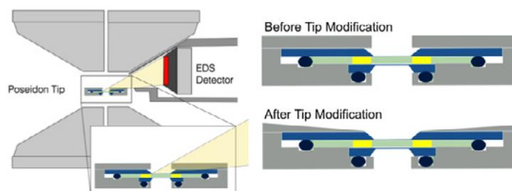
**Figure 7:** The left image shows the upper and lower pole pieces of a TEM objective lens. The EDS detector is situated just above and to the side of the sample holder. The yellow cone indicates the path the x-ray needs to take to be detected. With the current design, there is no line-of-sight from the sample to the EDS detector. The right shows the before and after modification to the holder tip. The holder lid has been modified to allow for line-of-sight.
