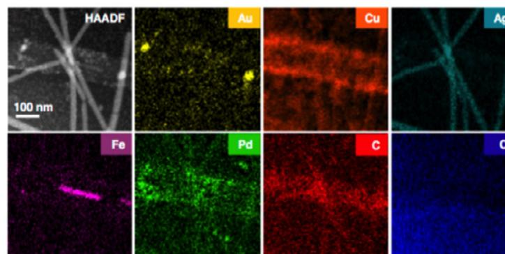
**Figure 10:** EDS spectrum image of a nanomaterial suspension consisting of Au and Pd nanoparticles, Cu ions in solution reduced by the electron beam, Ag nanowires, Fe catalyst and a multi walled carbon nanotube all in water.
